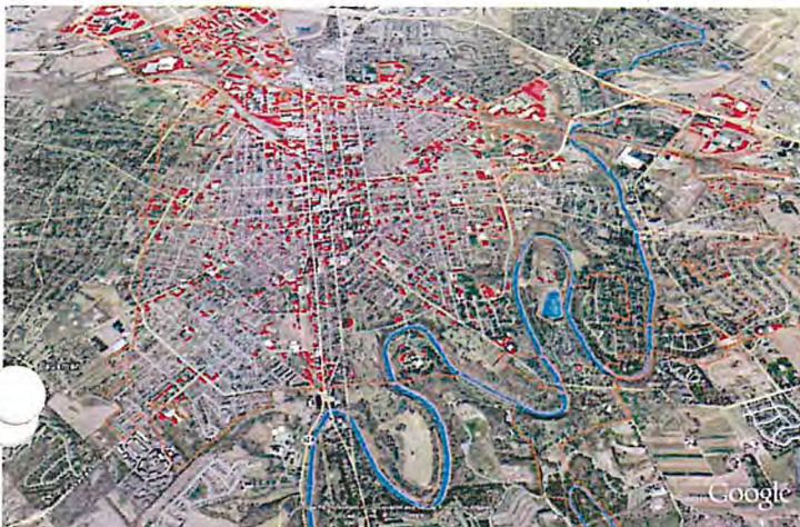
Lancaster, Pennsylvania is converting impervious areas such as parking lots (shown here in red) to permeable pavement within their combined sewer area. By using green infrastructure to infiltrate water on site, the city estimates they will reduce flows into their system by 700 million gallons – reaping over $600,000 annually in savings. Photo credit: City of Lancaster
